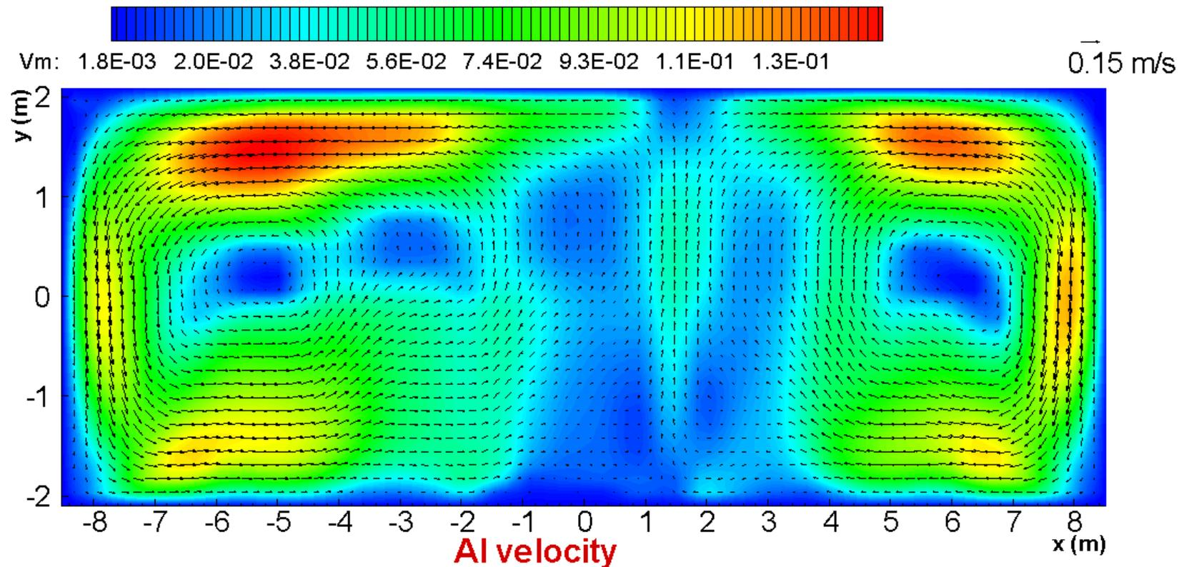
Steady-state metal pad flow velocity field
