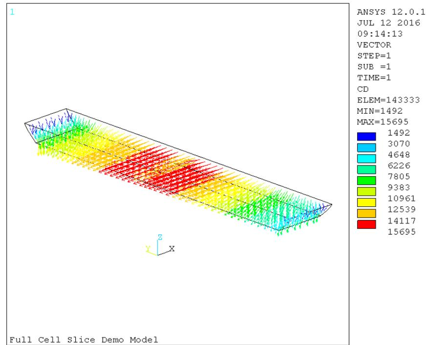
Thermo-electric model with current density in the whole domain (left) and in the metal pad only (right)
