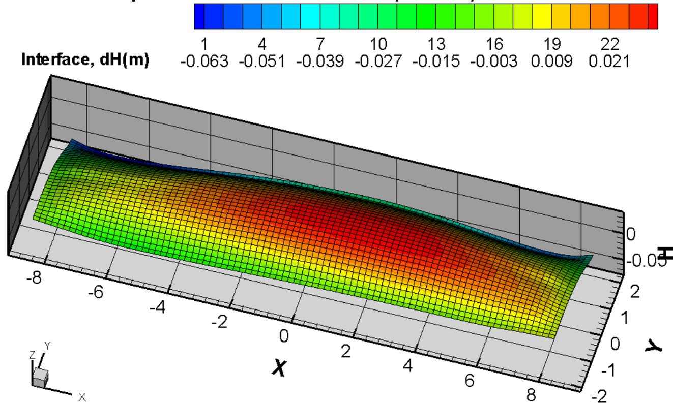
Steady-state bath-metal interface deformation
