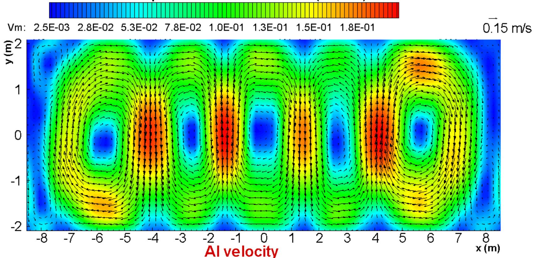
Steady-state metal pad flow velocity field
