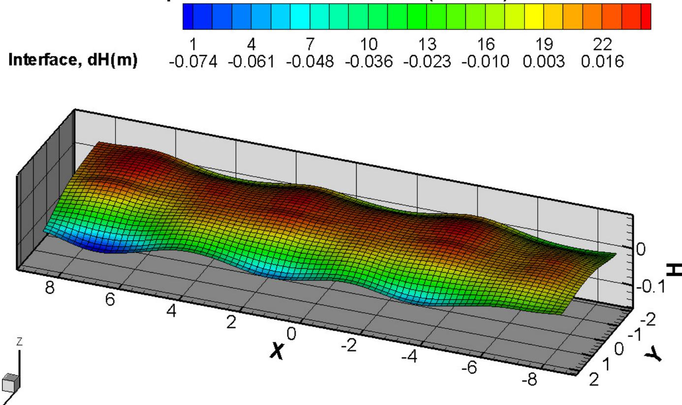
Steady-state bath-metal interface deformation
