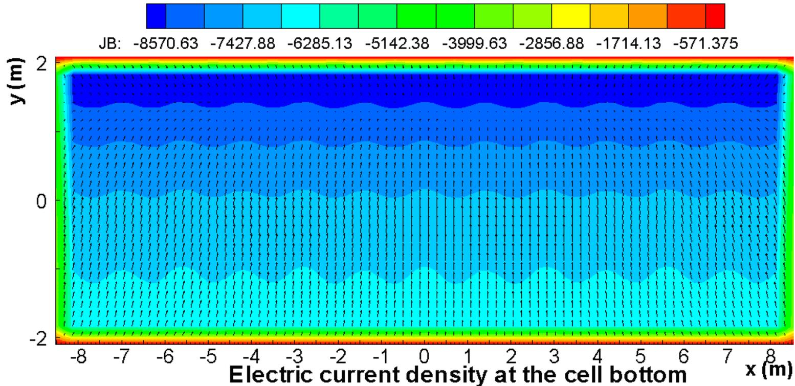
Current density calculated with MHD-Valdis. Contours: current density entering the cathode block. Arrows: Horizontal current density in the metal pad.
